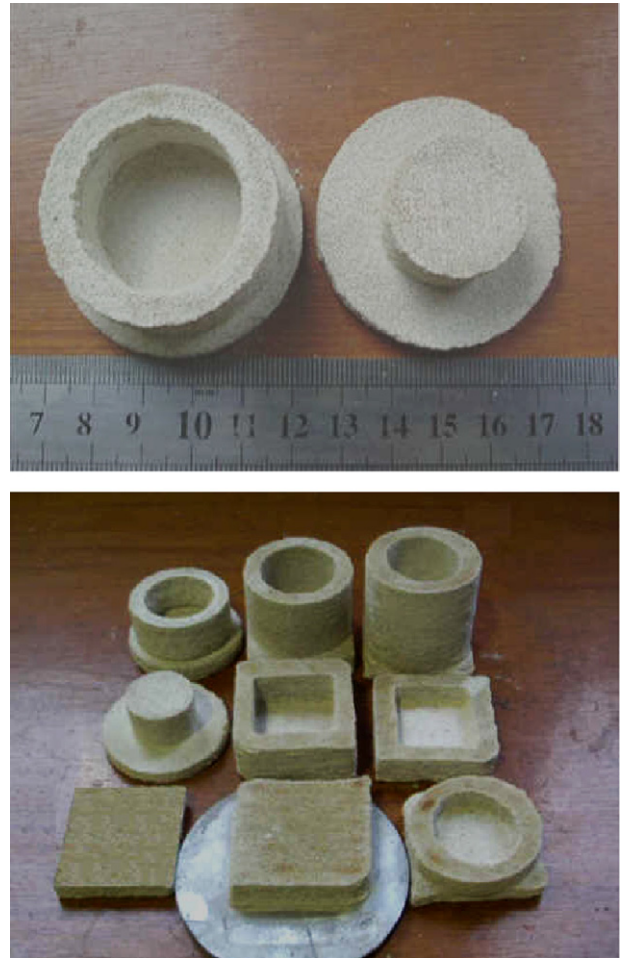
Fig. 5. Sand patterns sintered by selective laser sintering.
