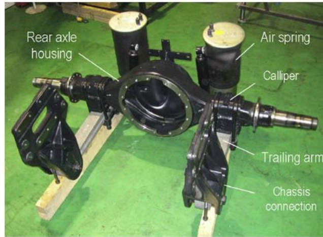
Fig. 1. Rear axle assembly of a commercial vehicle.
